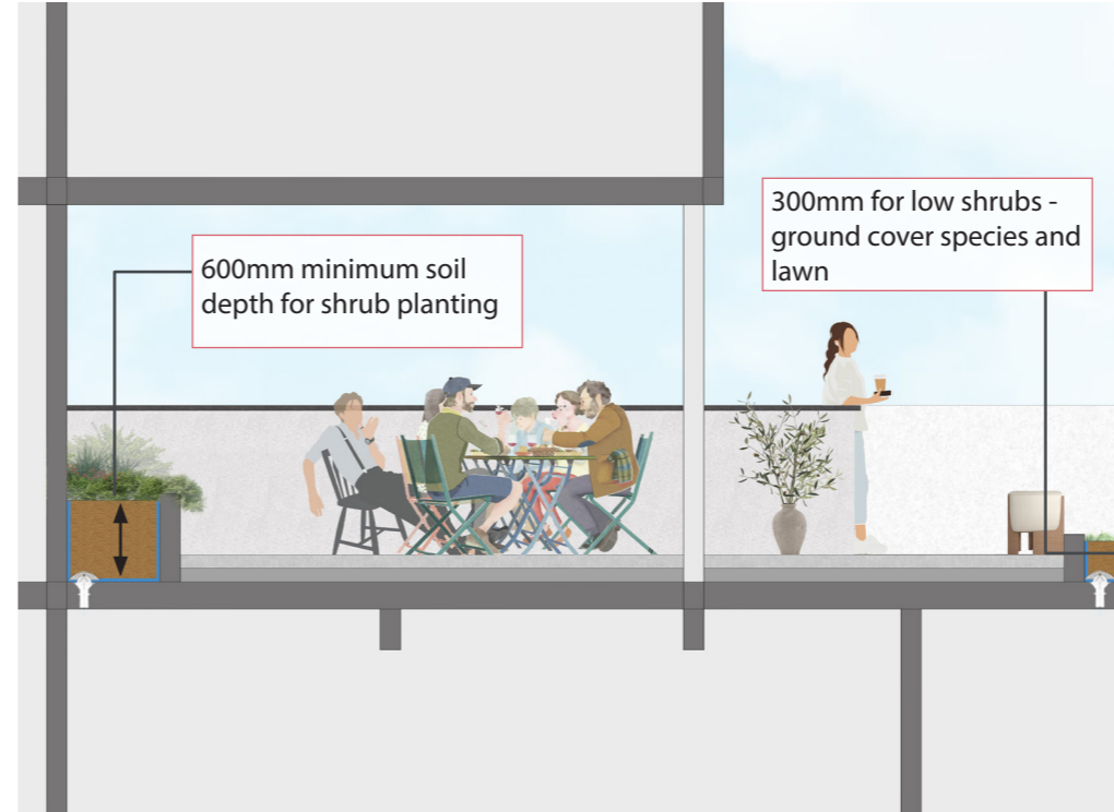
B2. Section showing the proposed climbing plant and ground cover planting (on structure)
